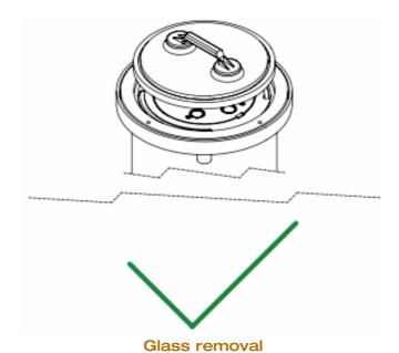
Use a suction cup to remove the glass to make any adjustments.
