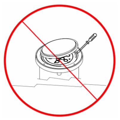
Do not use any tools to pry off, as this may damage the components and compromise sealing
