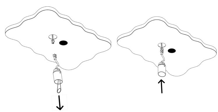
3 Remove the LED spot using the quick connector
