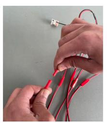
Remove the extension cable by taking off the quick connectors
